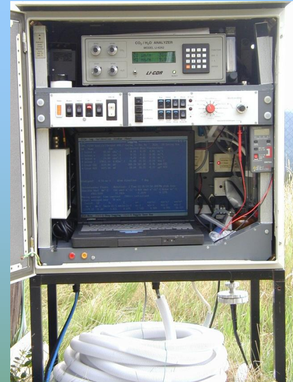
Infrared gas analyser and control computer
